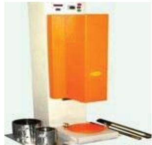
The machine is provided with a standard rammer weighing 2.6 kg for conducting light compaction and its weight can be increased to 4.89 kg for heavy compaction test by attaching additional rod supplied along with it. While using 100 mm dia mould the rammer carriage is locked in one position and the total area of the mould is compacted in about 25 strokes.
